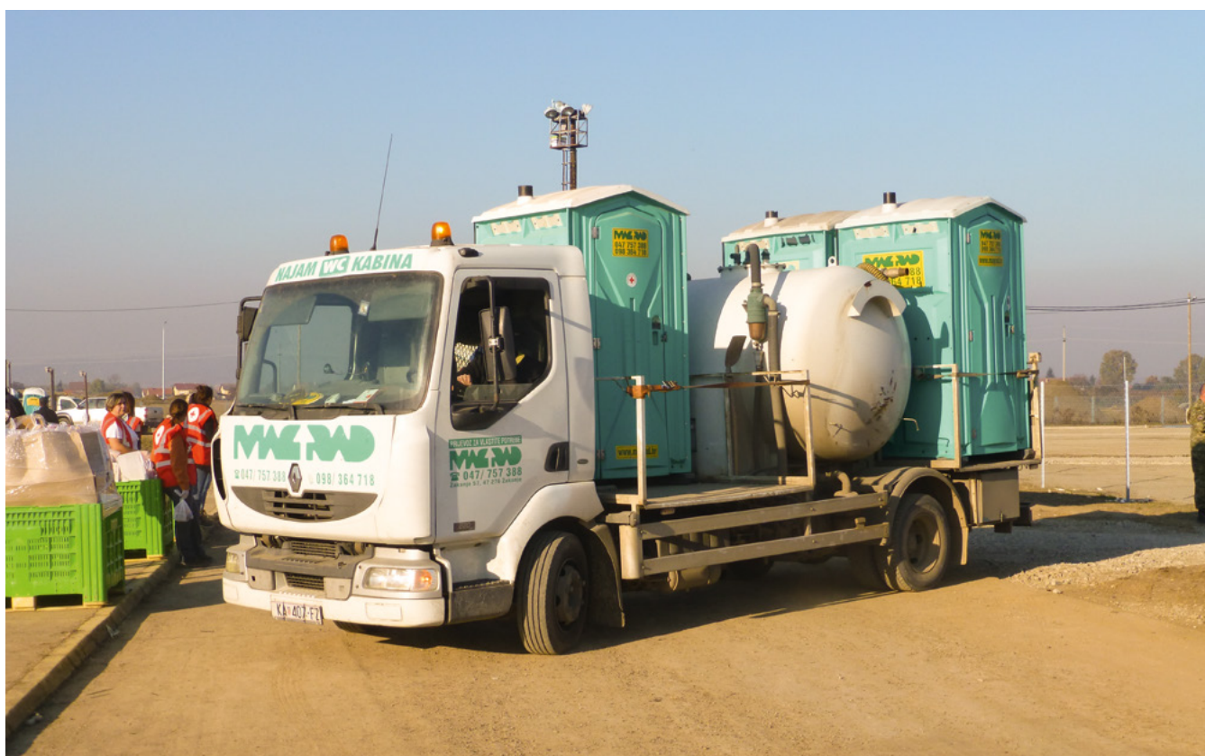
Desludging truck and portable, chemical toilets. Middle-East refugee crisis, Croatia. © Bünzli, 2015, SHA
